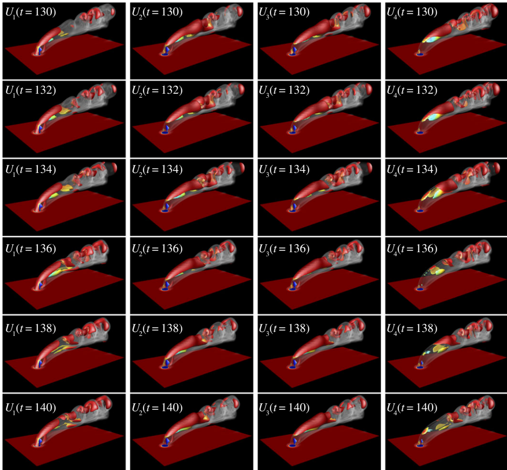
Figure 11. Snapshots of the OTD modes \mathbf{U}_i(\mathbf{x}, t) and the trajectory of the Navier–Stokes equations. Each row shows all four modes at a given time, with the first row taken at t = 130 . Time advancement from one row to the next is \Delta t = 2 time units. The modes are visualized by the iso-surface of the velocity magnitude equal to 0.02. The time-dependent base flow (DNS) is visualized by smoke volume rendering of a scalar field. (Online version in colour.)
