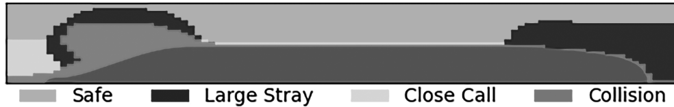
(B) Medium UUV operating envelope without N_{uv} compensation in sea state 6 at 90 meters deep.
