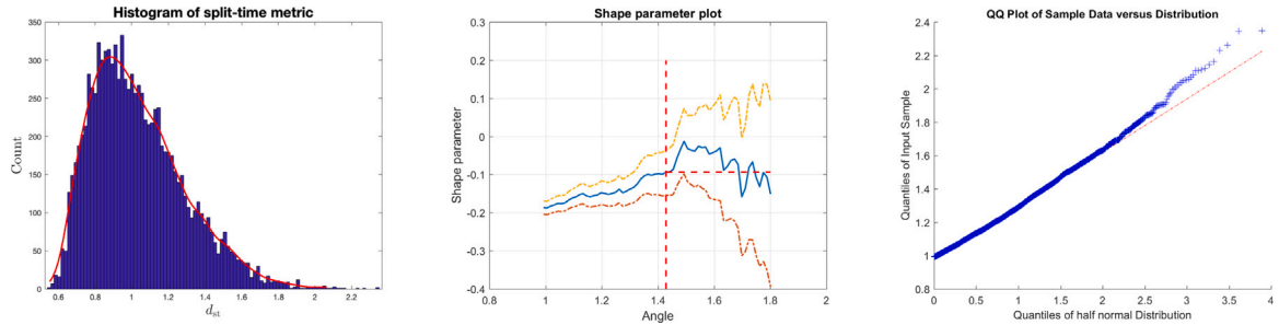
Fig. 9. The split-time metric from the Duffing oscillator: Left: histogram with a numerically estimated density; Middle: the shape parameter plot for the right tail; Right: the QQ-plot of the metric with the right-tail of a standard normal distribution.
